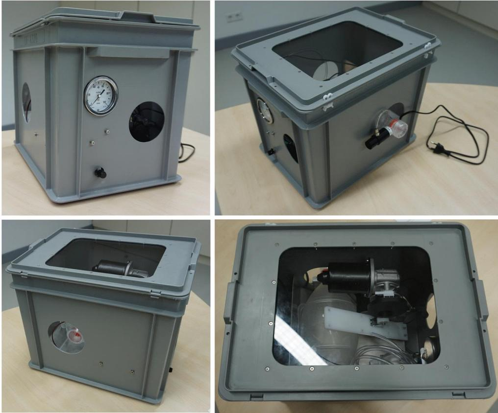
*4: Semi-automated resuscitator (TaBea), view of the prototype from different perspectives (without connected beathing tubes).*
